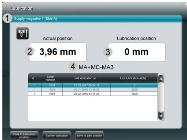
Fig. 34 Lubrication of the selected drive
