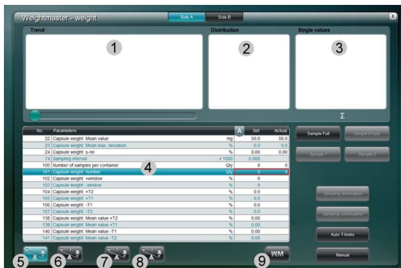
Fig. 36 Weightmaster graphic (Side A and B are only displayed at double rotary machines)
