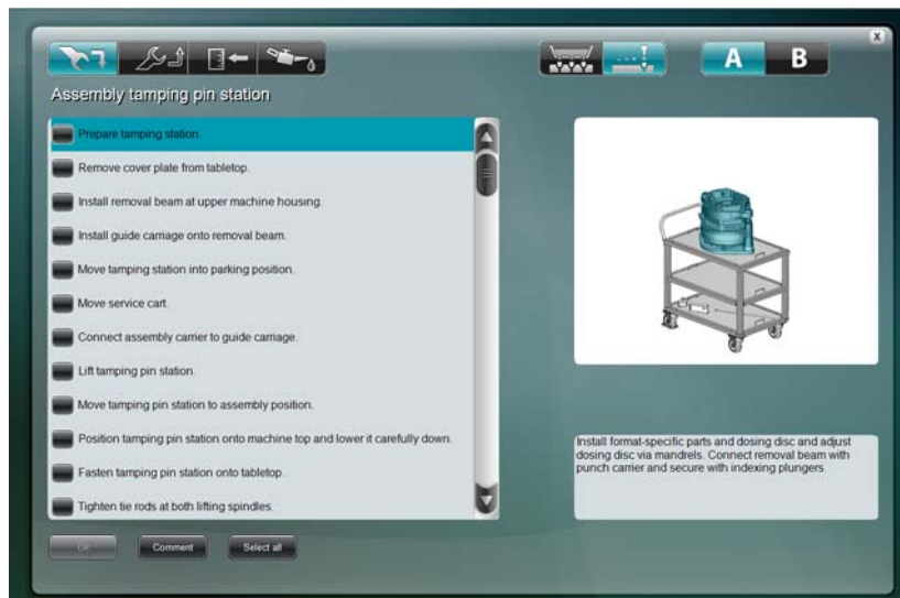
Fig. 28 Tamping station installation
