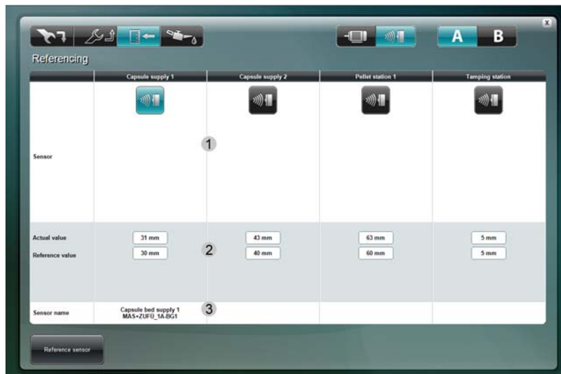
Fig. 31 Overview of all the sensors in the referencing overview
