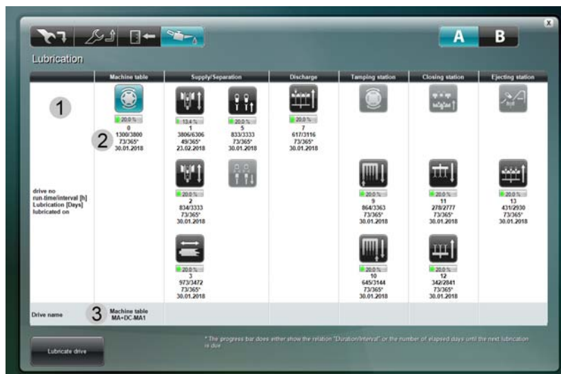
Fig. 33 Overview of all the drives in the lubrication overview
