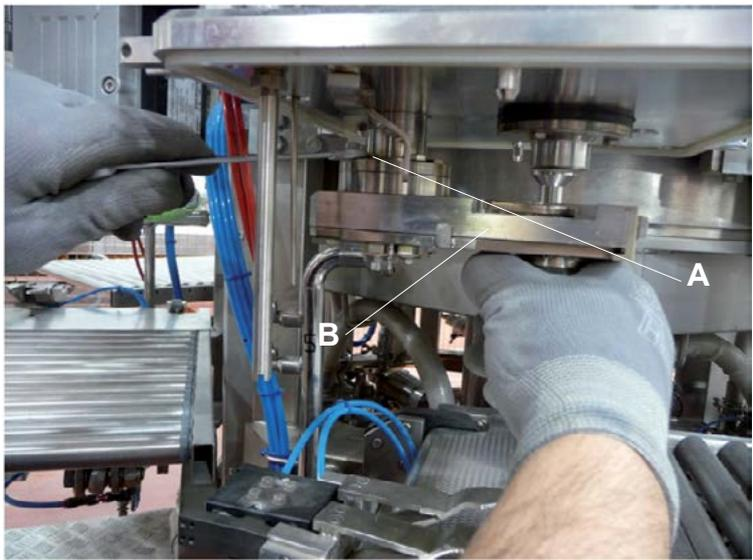
Unscrew the four bolts A which hold the uncapper plate B to the shaft. and extract it.
