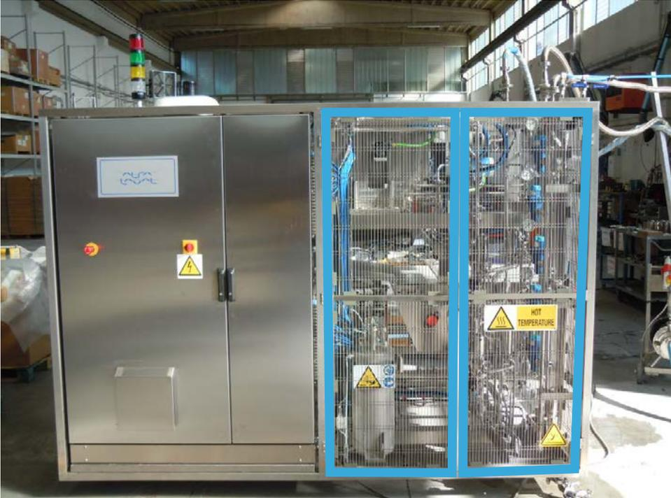
Stainless steel grid guards near the electric and pneumatic cabinets
