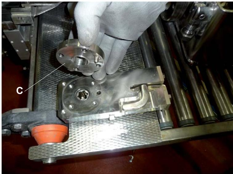
Remove the spacer C from the old clamping device.
