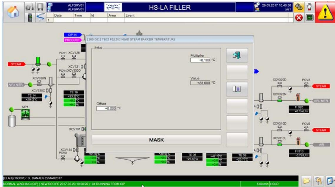
Clicking on each instrument field it is possible to see the Analogic Setup faceplate for the Analog Inputs.
