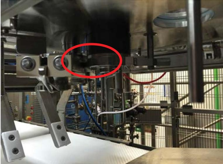
Push the e-stop and release the AX102 and AX105 brakes.
