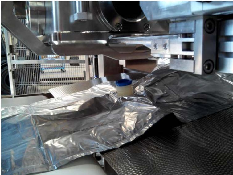
2. Once that the bag is released, pull out the bag strip from the bag loading area.
