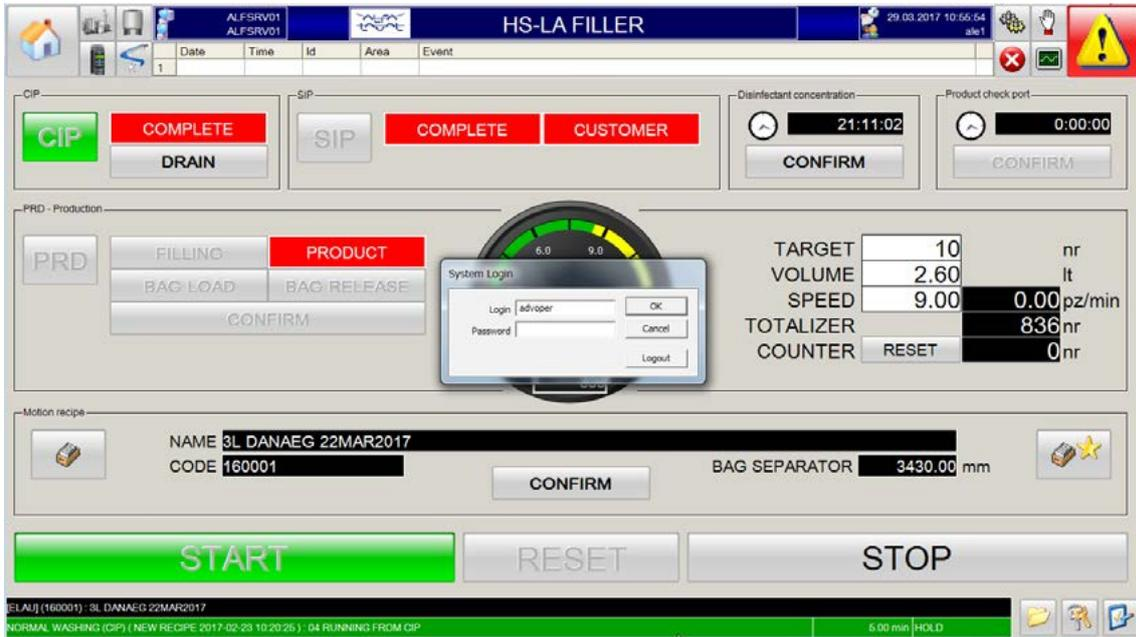
From this screen it is possible to login with different users. Each user has a specific array of access rights.
