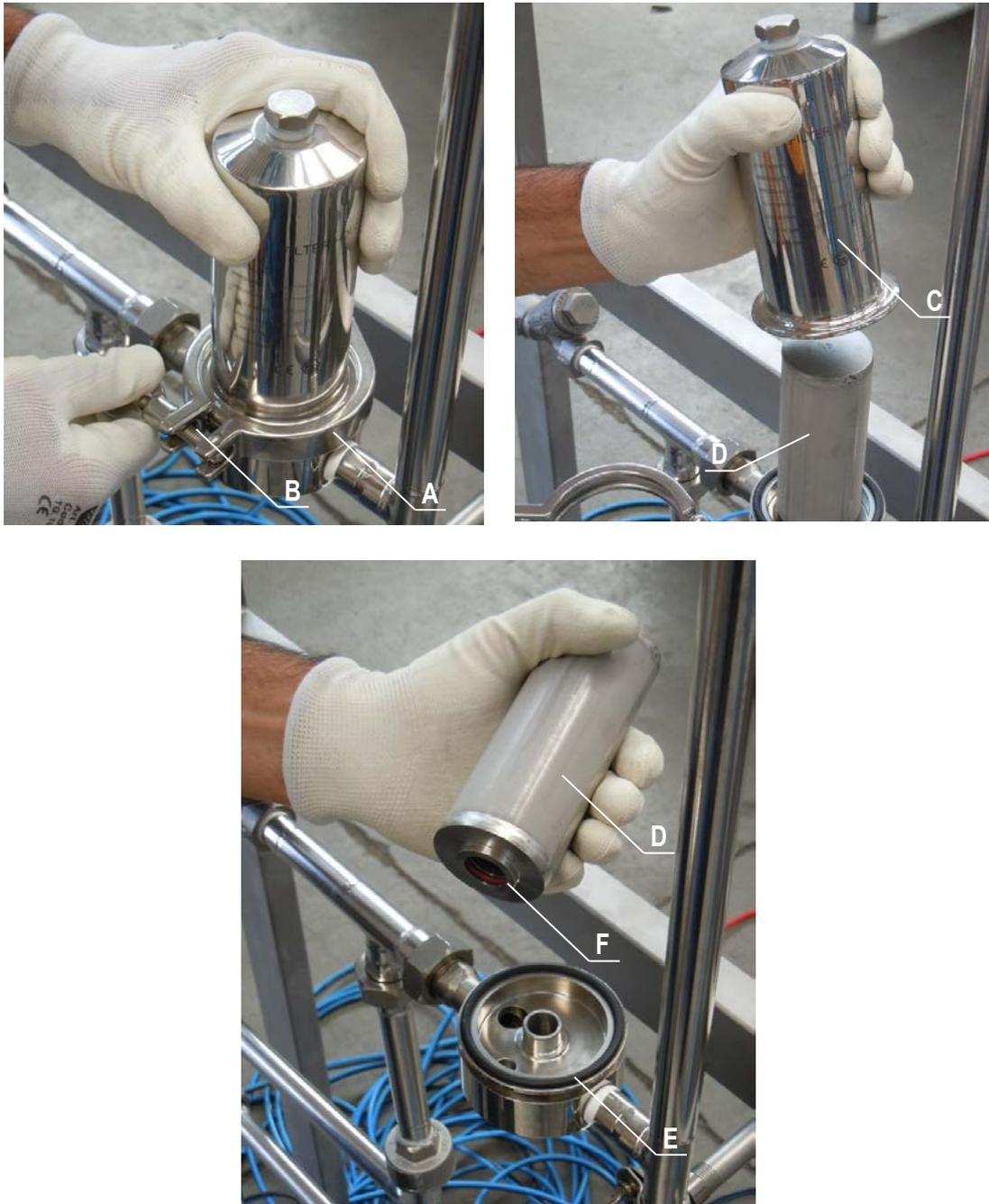
1. Open clamp A acting on screw B and remove it.
