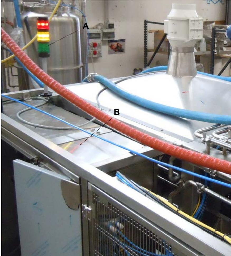
The machine may reach the customer with the luminous tower A disassembled, for transportation reasons. Restore the light tower A on the electrical panel B as shown in the top picture.
