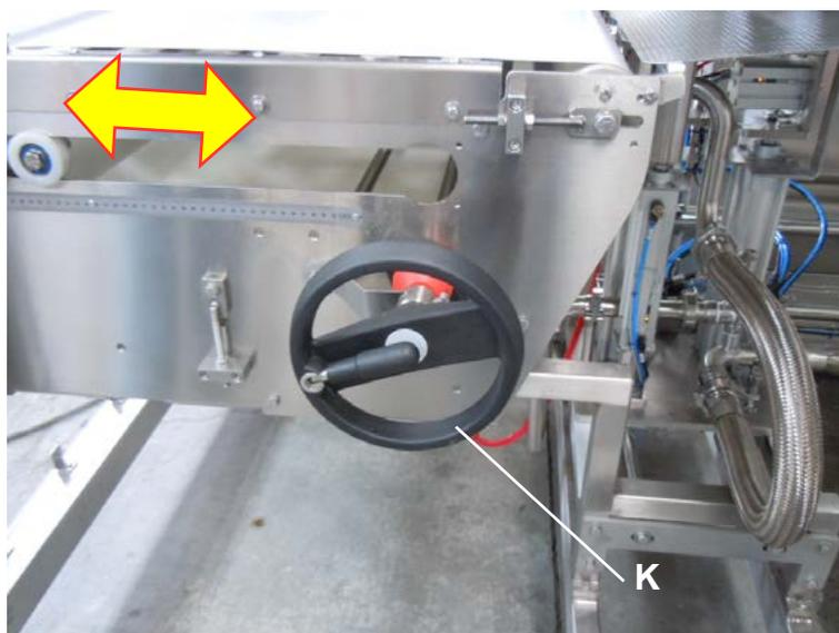
10. Adjust the position of the cutting unit by using the handwheel K, in accordance with the dimension of the first filled bag and the score line between the first and the second filled bag.
