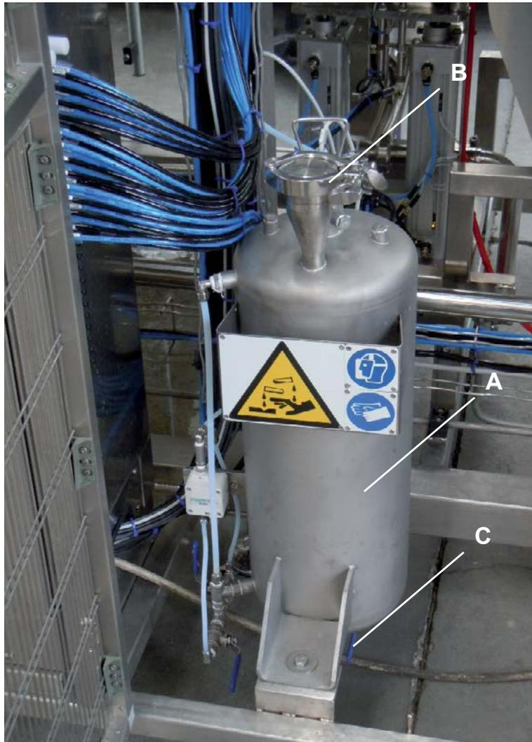
To load disinfectant in the tank A:
