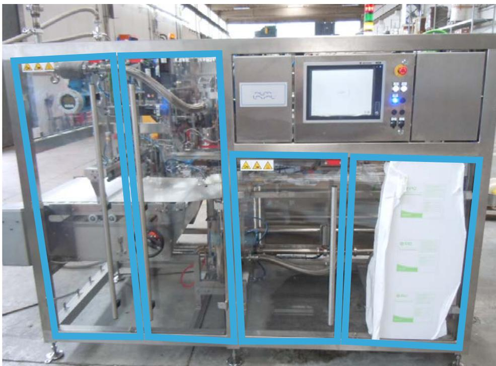
PVC guards in front of the operator area and the filling head area.
